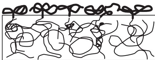
Figure 6.2: Modifying a surface using a diblock copolymer in which one block (thin lines) is the same as the substrate polymer, and the other block (rejected to the surface) has the desired amount of hydrophilicity or hydrophobicity.
