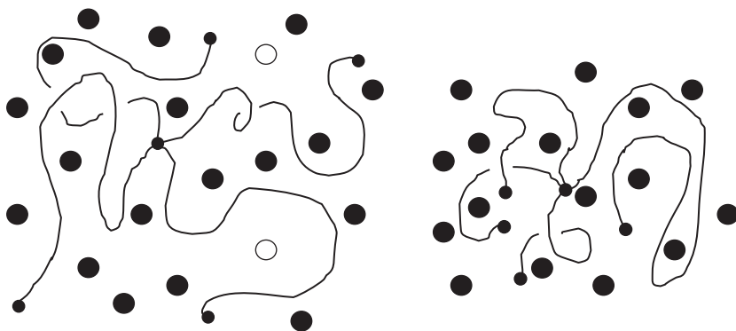
Figure 7.2: Typical configurations of four chains emanating from a tetrafunctional cross link in a polymer network. In the left sketch, the network was prepared in the undiluted state, and in the right sketch, it was prepared in solution and then dried. When a network is cross linked in solution and the solvent then removed, the chains collapse in such a way that there is reduced overlap in their configurational domains.
